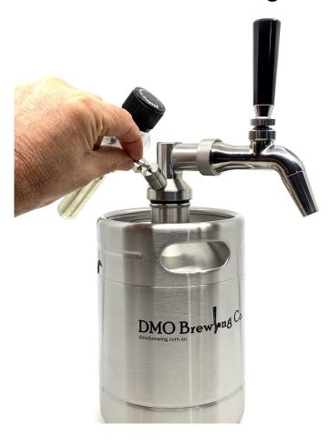
Pull on pressure relieving ring for a couple of seconds. If the keg was shaken in transit or warmed, it may contain excessive pressure which must be relieved before tapping. A hissing noise is expected.
