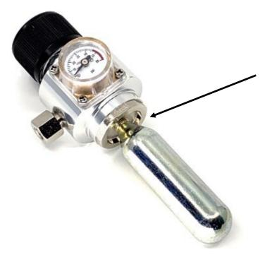
Turn in a new 16g CO2 Capsule with thread type of 3/8-24UNF, turn clockwise firmly into the regulator base.
